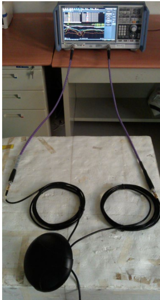
MA.673 antenna was tested with R&S ZNB-8 network analyzer.
