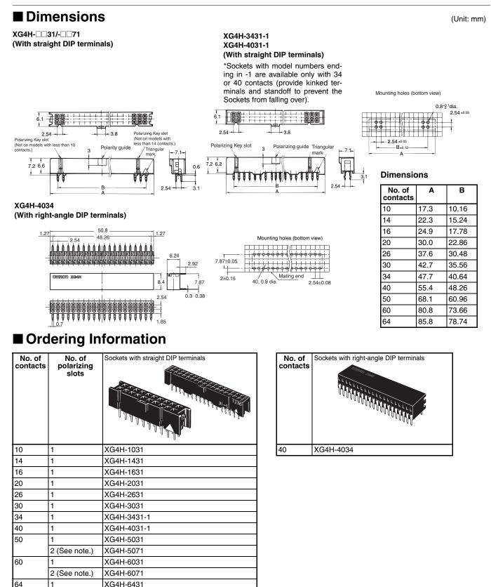
Note: Polarizing guide pitch is 22.86 mm.
